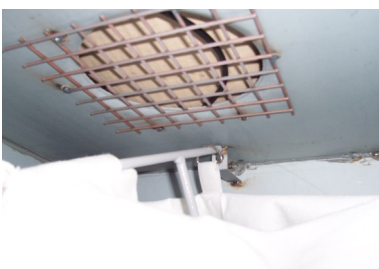
4. Remove shaker frame from rear support.
