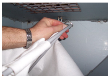
5. Remove rear retaining clip.
