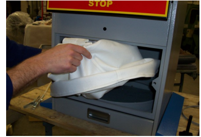
12. Remove dust filter.
