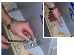
2. Release & Remove the transit bolts (see insert).
