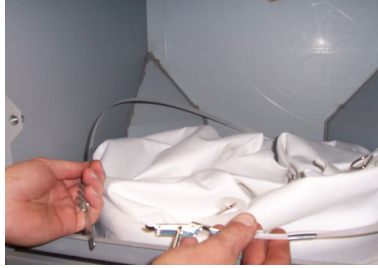
11. Remove retaining clip from extractor.
