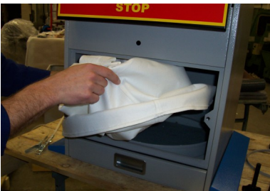
4. Fit dust filter over bottom seal.
