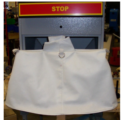
3. Ensure filter hanger and retaining clip are inline.
