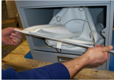
8. Remove shaker frame from dust filter.
