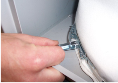
10. Release snap over retaining clip.
