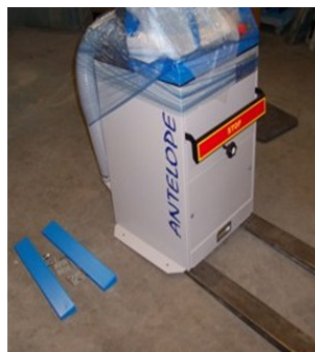
6. Slide the machine off the Fork Lift extensions onto the ground.
