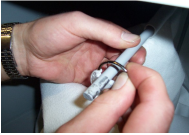
7. Remove front retaining clip
