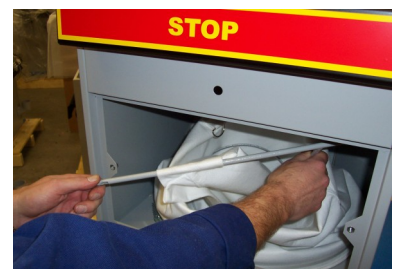
6. Remove shaker frame from extractor.
