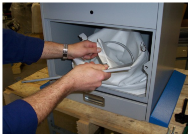
5. Re-assemble shaker frame & orientate filter hanger front to back of extractor.
