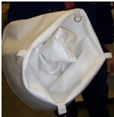
2. Fold dust filter inwards.
