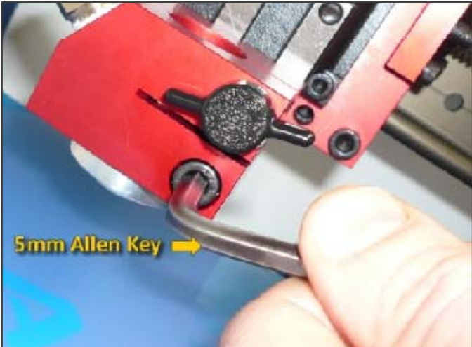
Loosen the cap screw and adjust the floating ring by turning until the tool tip protrudes...
