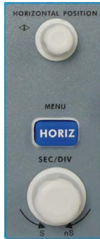
Fig. 4-12 Horizontal Control Zone
